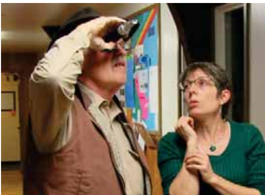
Francis Rothauge & Kelly Goodwin checking our member's honey moisture content with the refractometer.
